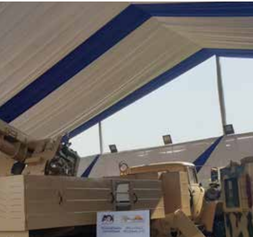
Egypt has proceeded with the integration of the Russian D-30 122mm howitzer mounted on a modified Ural-4320 6X6 truck chassis. The 122mm 6x6 Wheeled Self Propelled Howitzer can fire rounds out to ranges of 15.3km with standard ammunition and 21.5km with base bleed ammunition.
